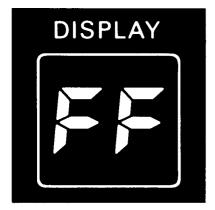
This flashing code tells you to check your frozen food. Has any of it started to thaw? A package may be holding the freezer compartment door open. Don't open the door more often than absolutely necessary while this code is displayed. Touching the STATUS CHECK-RESET pad after the freezer compartment temperature has returned to normal will erase the code.
